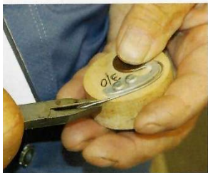
Bending the hook to shape on the jig.
