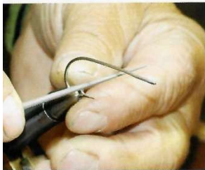
Tapering the hook shank and refining the point, barb and gutters.
