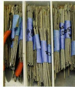
Wires cut to size.
